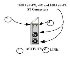
The module is equipped with an Activity (A) LED, and a Link (L) LED which indicates proper connectivity with the remote device when lit. Lettering on the front of the module identifies it as "100 FX" to avoid confusion with other similar-looking FPMs.
